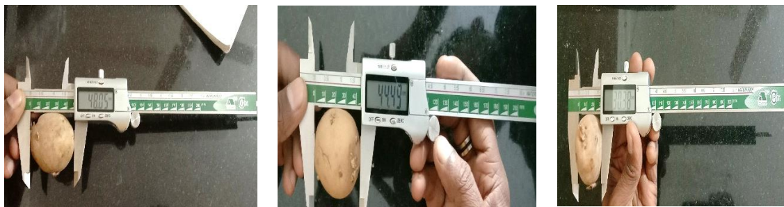
Fig.1 Measurement of maximum, intermediate and minimum diameter of round shapes
